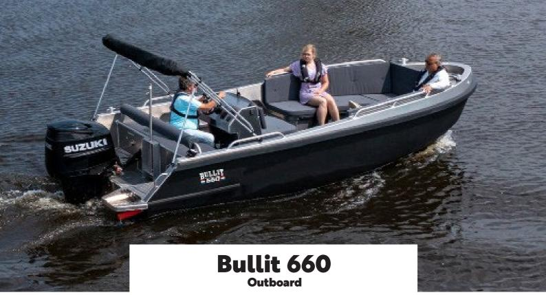
The Alumax Bullit 660 Outboard is an undisputed lightweight. The light aluminium tender has remarkably little draught and has excellent sailing characteristics and unprecedented stability. The Bullit 660 can safely remain in the water in winter and freeze if necessary.
