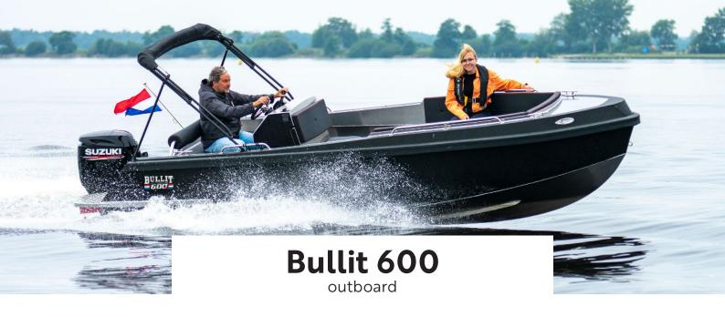
The Alumax Bullit 600 outboard is an undisputed lightweight. The aluminum tender has remarkably shallow draft and has excellent sailing characteristics and unprecedented stability. The Bullit 600 can be left in the water in winter and freeze if necessary. Every Bullit that leaves the Alumax yard, is hand-welded. Even the installation of technology and finishing are purely manual. Production is flexible, allowing us to provide customization.
